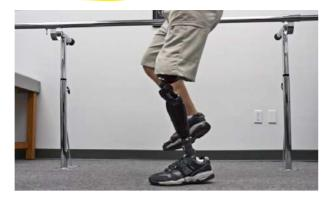
When the knee is flexed, loaded, and is stationary for a preset period of time (3/4 to 3 seconds), flexion will be automatically locked until it is extended. With ALLUX 2, Safety lock function has been improved to include a vibration from the knee-joint, letting the user know Safety lock has been engaged.
