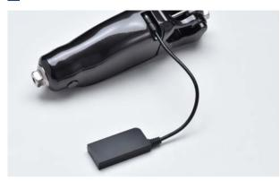
ALLUX 2 battery life is approximately 4 days (5000 steps/day on prosthetic side). The charge time for an empty battery is only 3 hours and a Backup battery is included in case of emergency.
